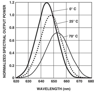
Figure 6. Typical Spectra Normalized to the 25° C Peak.
