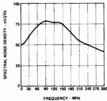
Figure 12. Typical Output Spectral Noise Density vs. Frequency.
