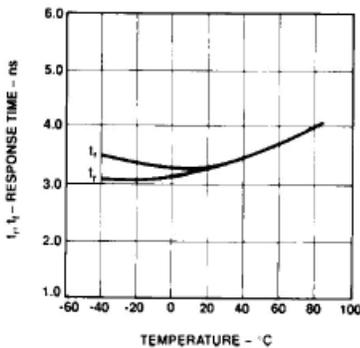
Figure 13. Typical Rise and Fall Time vs. Temperature.
