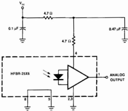
Figure 9. Recommended Power Supply Filter Circuit.
