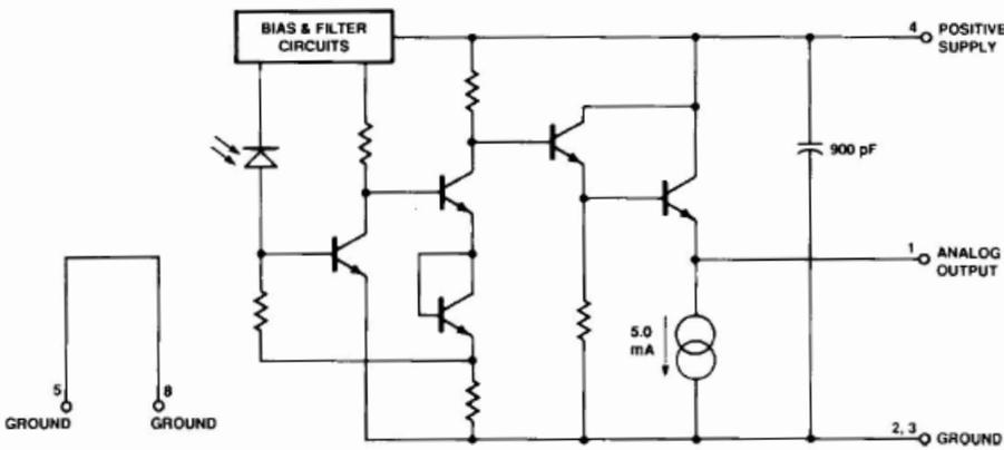
Figure 10. Simplified Receiver Schematic.
