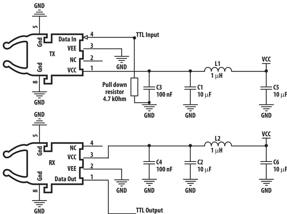
Figure 2. Recommended Transmitter and Receiver Application Circuit
